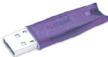
to the eToken line of Internet security solutions, following the eToken R2 USB-key first released last year which featured an advanced DESX 120-bit encryption engine.
